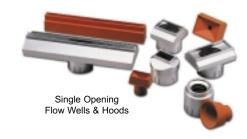
Wave configuration is a critical factor. Flow Wells determine the solder wave, which matches the component lead pattern. The solder flow can be accurately directed away from adjacent components to limit heat exposure to sensitive areas. The corresponding Air Cleaning Hood directs low pressure air against the lead pattern, forcing molten solder to drop from the holes into the empty Flow Well.
